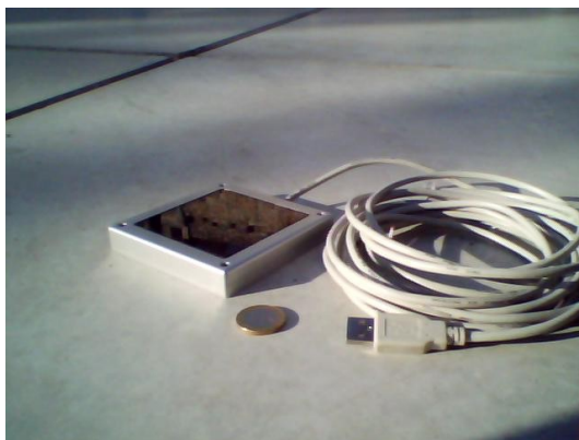
Lightmeter and USB-cable compared to 1 Euro coin.
