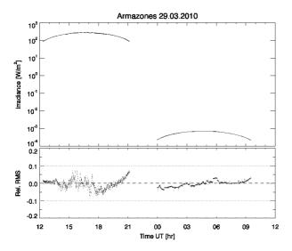
Fig. 2. Example of a fit of the measured LIGHT-METER data to the irradiance model for March 29th, 2010 (no clouds were present, night with full moon). The relative RMS (lower plot) of the fit between the measured data and the irradiance model inside the range of 10%. Because of the good fit performance the measured data are not distinguishable from the computed irradiance model.
